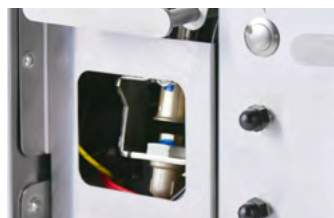
Spark generator supplied with 230 V
